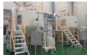
• Disc type, Φ120mm, 1500rpm • Φ2600 mm, Max Temp. 250°C
