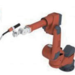
Robot Mechanics Classic Wrist with Enlarged Operating Range by 7th Axis
